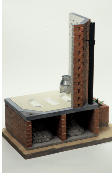
Figure 2.3 and 2.4: Compost toilet with dual chamber, urine separation and ventilation
