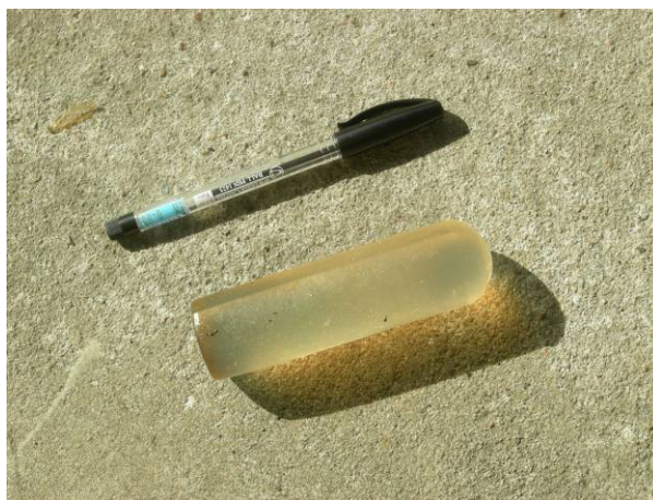
Figure 6.13 Filter which is put in the overflow pipeline (the pen is included in the picture to show the size of the filter)
